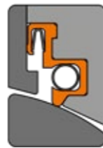
Valve seal with several spring-loaded sealing lips, for example once against the valve and once against the housing.
