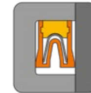
Encapsulated v-spring for sealing without dead space or against very aggressive media
