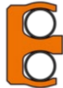
With two grooves manufactured seal for special dimensions or large groove dimensions
