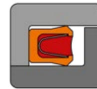
Seal with filled spring chamber for sealing without dead space in food products
