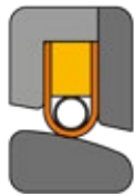
Valve Seal with encapsulated coiled spring for dead space free sealing. Support ring can be made of metal or plastic, depending on the application.
