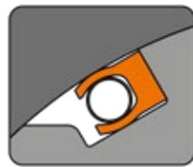
Ball valve seal. Tilted sealing profile integrated into the ball.
