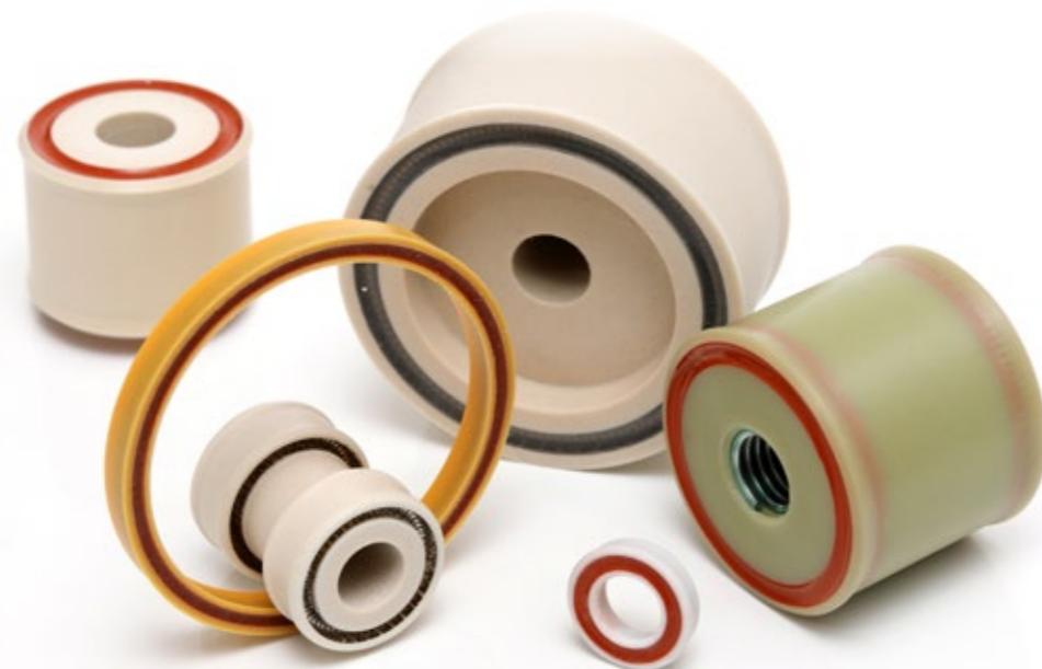
Special solution v-packaging. Sealing system consisting of several parts, such as a spring energized seal and support rings, to enable sealing at very high pressures such as over 1000 bar
